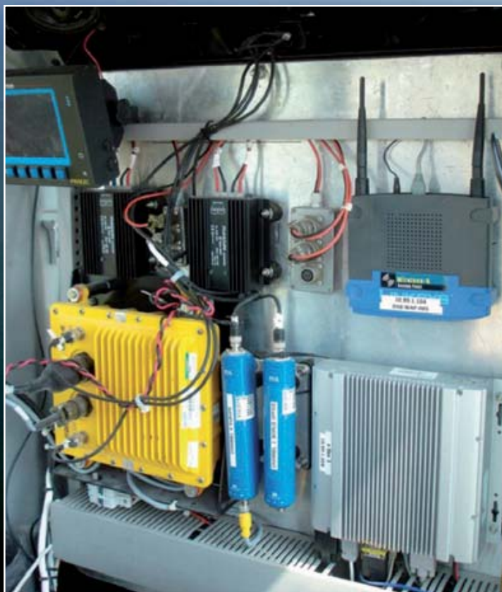
Pacific Crest's machine control product, Sitecom, is installed in Van Oord dredgers to enable high-precision GPS locating and tracking.
